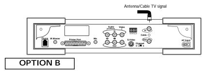
If you have a standard coaxial cable type of antenna or a Cable TV signal, use this option.
